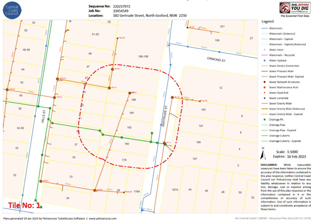
Figure 4 Council Asset Plan showing location of pits and pipes to which the easement relates.
